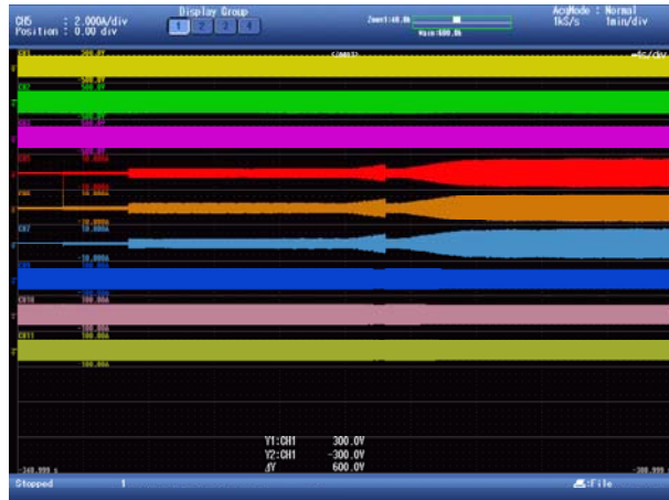
Figure 13 Photovoltaic Grid - Connected Steady Process Voltage Current and Grid - Connected Current Variation Waveform.
