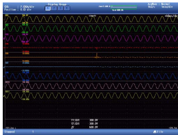
Figure 12 Photovoltaic grid - connected instantaneous voltage and current and grid - connected current changes waveform.
